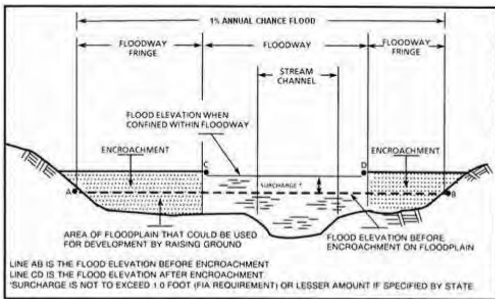
FIGURE 2 – Floodway Schematic
